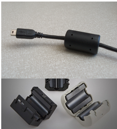
Figure 31: Practical examples of ferrite beads
